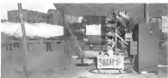
The J45—three shafts from a modified J-4 engine in the thrust plate of an early G-4 test run. The jet produced 1250 pounds thrust, weighed 700 lbs.
